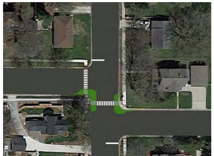
Recommendations A. Mantorville Ave and 7th Ave NE. Current (left) and recommended (right). Curb extensions, high visibility crosswalks and advanced stop bars provide increased safety and improved visibility at an intersection with high pedestrian volumes.
