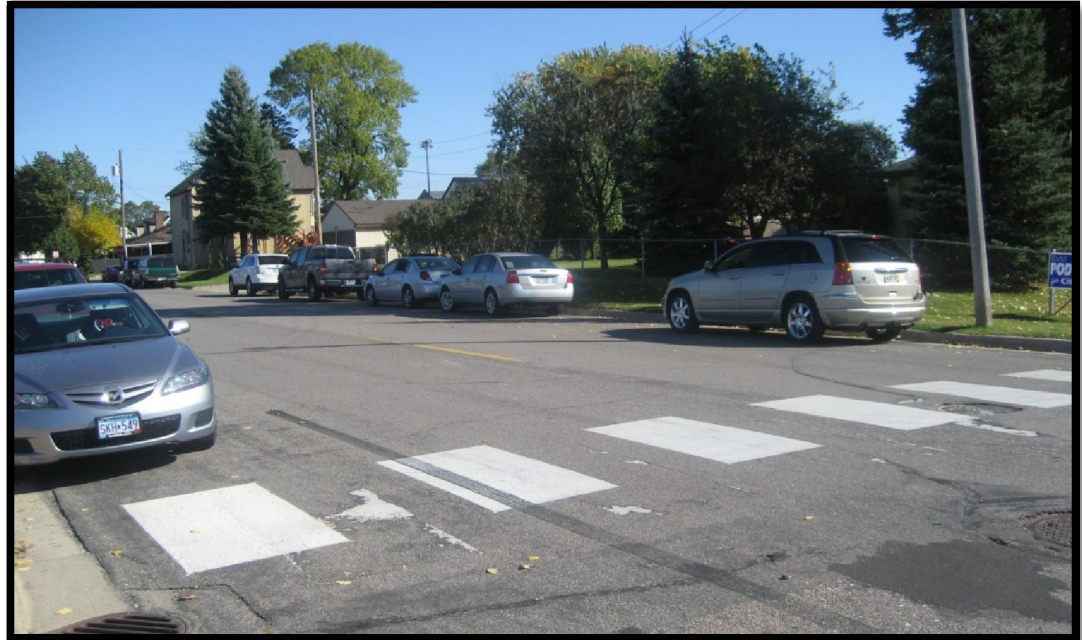
Vehicles parked on 3 rd Street N up to the crosswalk at 10 th Avenue. The parked vehicles limit the visibility of pedestrians as they step off the curb to cross.
