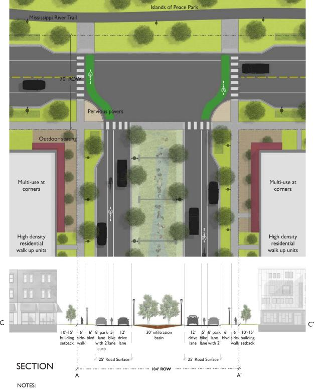
Street light spacing 100' Pedestrian light spacing 50' Tree plantings staggered spacing 45'
