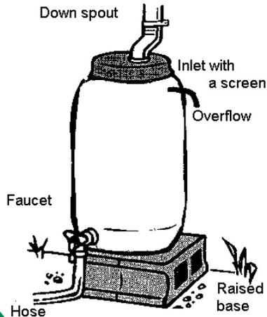
**Capture:** A rain barrel captures water from roof downspouts. Even small roofs and rainfalls can easily fill a 55 gallon rain barrel. When the rain barrel is full, water overflows through an overflow pipe.
