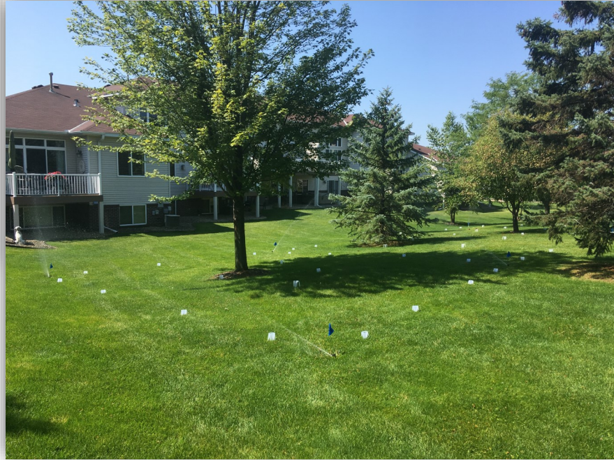
(Below) Water in Motion staff assemble catch cans for distribution uniformity test.
