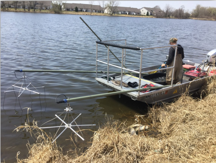
(Above) The electrofishing boat temporarily stuns fish, allowing them to be collected for analysis.
