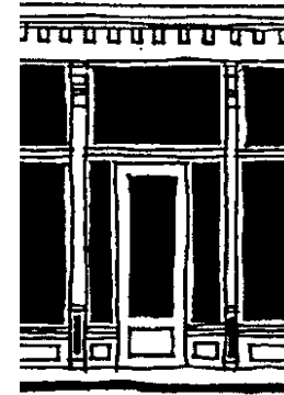
Original storefront doors were typically recessed, constructed of wood with a large window above a single or double panel that complemented the bulkhead design below the display windows
