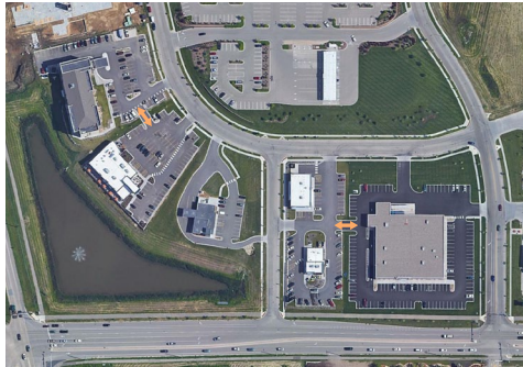
Providing cross access to adjacent businesses reduces traffic and the potential for crashes on roadways.
