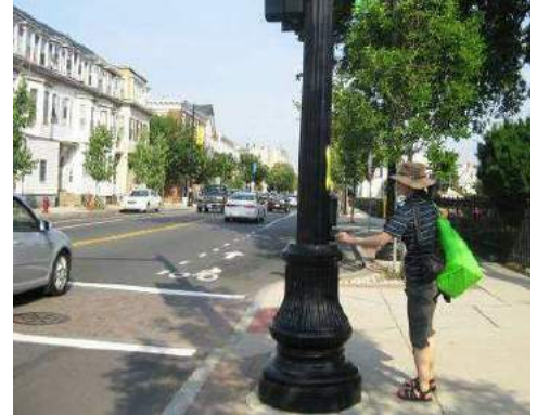
Pedestrian push buttons must be in a location accessible to people walking and using mobility devices.
