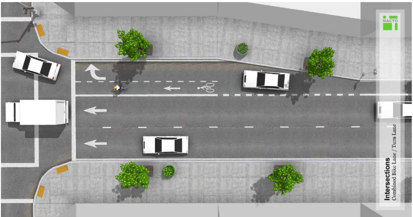
Combined bike lane/turn lane recommendations from the NACTO Urban Bikeway Design Guide
