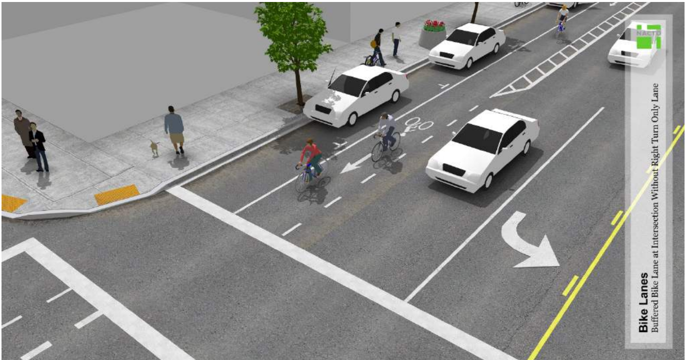
Buffered bike lane intersection recommendatiosn from the NACTO Urban Bikeway Design Guide
