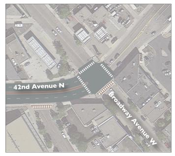
Proposed - Alternative I: A limited approach includes a pedestrian refuge median on the southwest crossing and slight reduction in lane widths.
