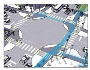
A rendering of protected intersection for bicyclists. Elements such as advance vehicle stop bars, corner refuge islands, setback bike crossings, and bicycle-specific signals are included in this concept. Image courtesy of protectedintersection.com
