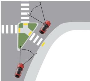
Two different slip lane configurations: the first prioritizes vehicle speed, the second improves pedestrian safety while also improving driver sight lines.
