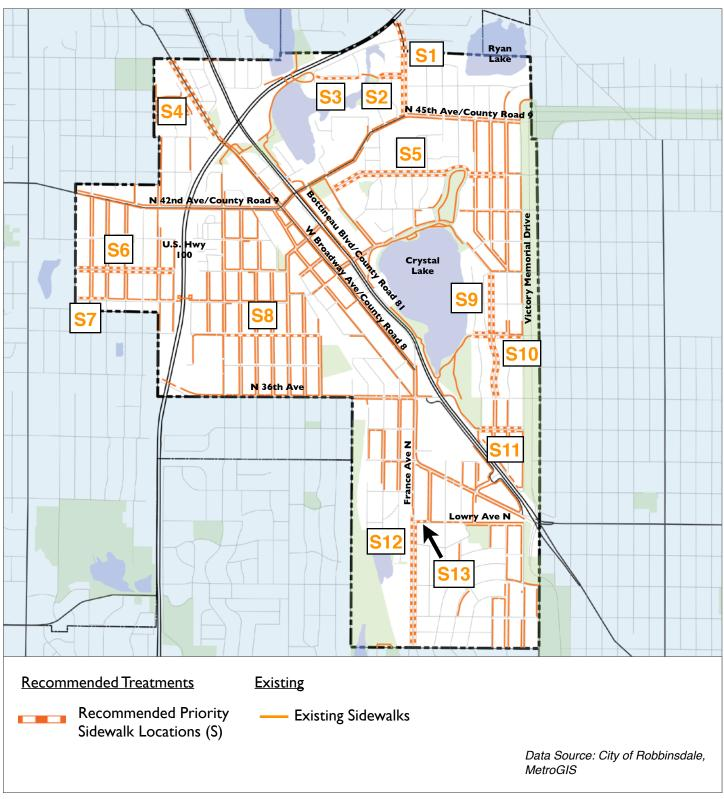
Recommendation: Install 5 foot minimum sidewalks where missing. The city has a plan for filling sidewalks gaps.
