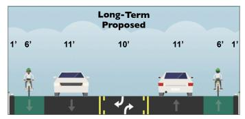
Proposed configuration 2: Narrower travel lanes calm traffic and create space for a painted buffer for the bike lanes.
