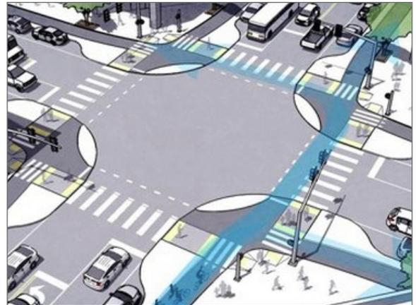
**A rendering of protected intersection for bicyclists. Elements such as advance vehicle stop bars, corner refuge islands, setback bike crossings, and bicycle-specific signals are included in this concept. Image courtesy of [protectedintersection.com](http://protectedintersection.com)**
