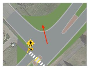
By reducing the vehicle turning radius, the speed of turning motor-vehicles is reduced and the street becomes more comfortable for pedestrians and bicyclists to cross.
