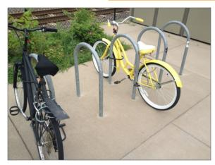
Inverted-U style bicycle parking should be installed at key destinations close to the primary entrance to the building.
