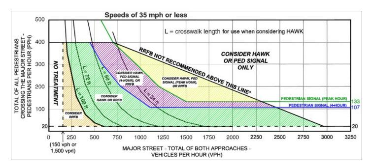
5.2.2.c - Guidelines for the Installation of Pedestrian Hybrid (HAWK) Beacons, Pedestrian Signals, or Rectangular Rapid Flash Beacon (RRFB) Signs on High-Speed Roadways from the City of Boulder Pedestrian Crossing Treatment Installation Guide
