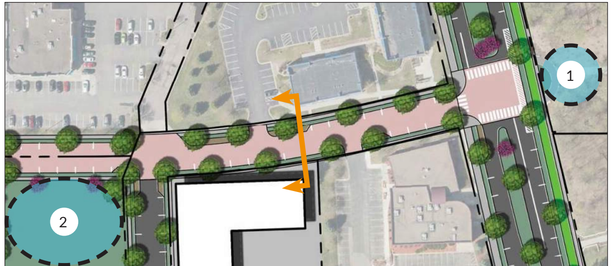
Figure 67. Conceptual design of 35th Avenue N as a managed street connecting the Hilde Performance Center (labeled "1") to existing restaurants and future redevelopment around City Center Green public space (labeled "2"). Orange line with arrowheads indicate the approximate location of street cross section, figure above.
