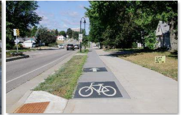
▲ Curb separated directional (one way) cycle track adjacent to sidewalk. (Richfield, MN) When placed adjacent to the sidewalk, a detectable surface should be placed at the edge of the bike lane for people with vision impairments.
