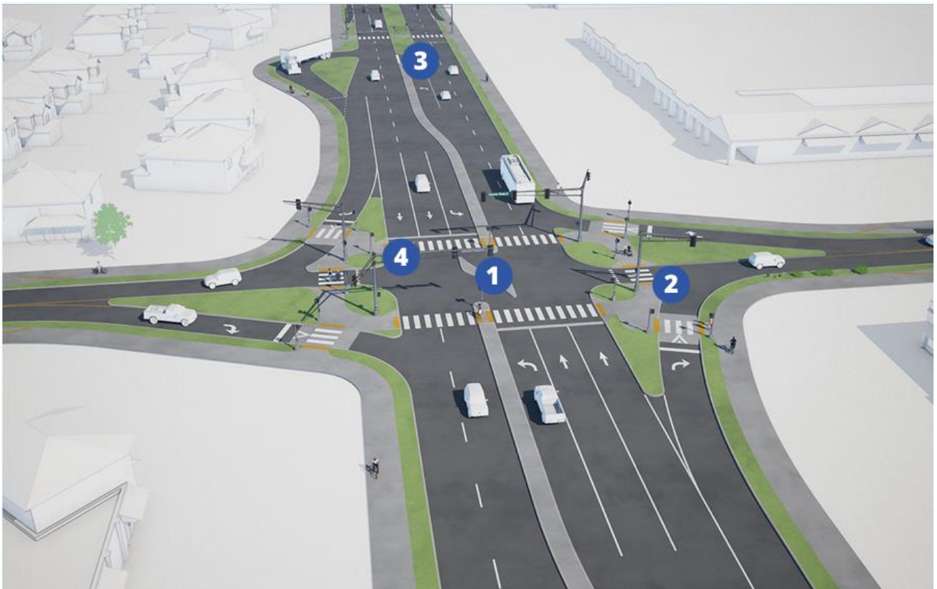
A protected intersection can provide a crossing option in areas with high traffic and speeds. Image courtesy of Federal Highway Administration's " Improving Intersections for Pedestrians and Bicyclists. "
