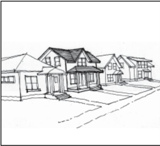
Appropriate infill: Roof forms, height, and detail are compatible.
