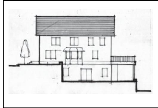
Inappropriate: Clearing the site; using cut and fill and retaining walls.
