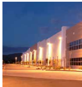
Exterior lighting should use full cut-off fixtures that prevent light trespass and glare, especially as seen from the marsh
